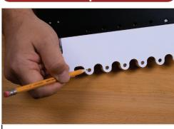
With the stock still secured to the jig, flip the jig over and mark the stock using the template as a marking guide.
