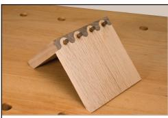
Assemble the joints as shown in your Fast-Joint instructions. Now, apply glue to dowels (not included) and insert them into the holes that were just drilled.
