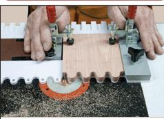
Complete the male cut with the Fast-Joint jig.
