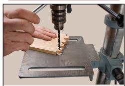
Aligning the drill bit with the holes, drill your stock about half way in. Do not protrude out the back side. Note: You may want to use a depth stop to prevent accidentally drilling all the way through the stock. Go to www.ptreeusa.com for more unique Fast-Joint templates and accessories
